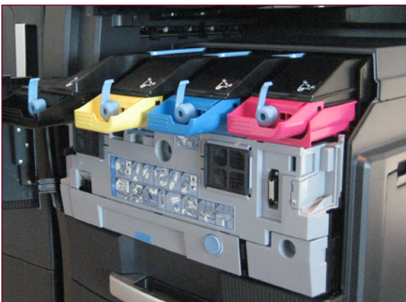
Each toner cartridge has a release lever that users lift up to pull out the cartridge as well as a handle for easy carrying
